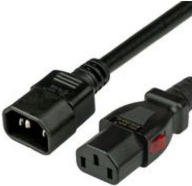
IEC 60320 C14 C13 LOCKING Power Cords are commonly used in environments where high availability is critical. The locking C13 connector ensures that the connector never detaches from inlet.
