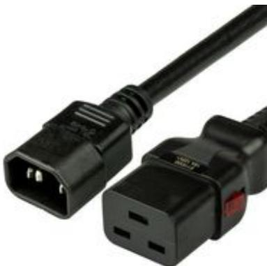
LOCKING IEC 60320 C14 to C19 Power Cords feature a locking mechanism on the C19 (female) end of the cable. C14 to C19 locking power cables are used in data centers and for critical OEM equipment to protect against accidental disconnects and to ensure a secure connection.
