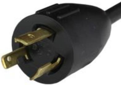
The NEMA L5-20P is a 3 Wire grounded plug with a hot, neutral , and ground pin rated up to 125V and 20A. This plug can be locked into place on the matching receptacle which prevents nuisance disconnection. This plug looks nearly identical to L5-30P but is slightly smaller in pin thickness and alignment circumference. Refer to either plug, receptacle or face plate to find out your amp requirements.
