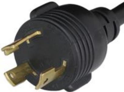
The NEMA L5-30P is a 3 Wire grounded plug with a hot, neutral and ground pin rated up to 125V and 30A. This plug can be locked into place on the matching receptacle which prevents nuisance disconnection. This plug looks nearly identical to L5-20P but is slightly larger in pin thickness and alignment circumference. Refer to either plug, receptacle or faceplate to find out your amp requirements.
