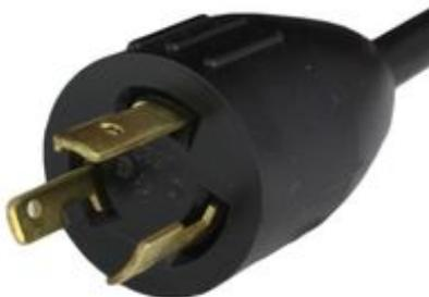
NEMA L5-20P (TWIST LOCK) Power Supply Cords are rated up to 125VAC and 20A. These power cords are available with IEC 60320 C-13, IEC 60320 C-19, NEMA 5-20R (STRAIGHT), NEMA L5-20R (TWIST LOCK), NEMA 5-20R (STRAIGHT), and other connectors (receptacles). Standard jacket type is SJT(OW) but rubber cordage is available. Other jacket colors (white, gray, blue, green, red, yellow, orange) are available.
