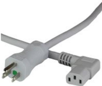
We currently stock Grey Hospital Grade NEMA 5-15P to right angle IEC60320 C13 in 5 meter lengths. Plugs, Connectors and Power Cords used in medical applications must have a green dot clearly displayed on the housing surface to show conformance with Underwriter Laboratories specifications UL817, UL60601-1 and UL498. It states in UL60601-1 that all patient care equipment must use power cords with hospital grade attachment plugs.
