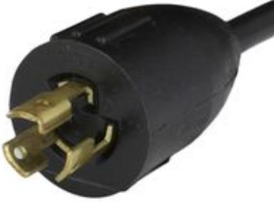
The NEMA L5-15P is a 3 Wire grounded plug with a hot, neutral and ground pin rated up to 125V and 15A. The plug can be locked into place on the matching receptacle which prevents nuisance disconnection. This feature makes this plug popular in commercial and industrial settings where high traffic or moving of equipment is common. This plug can be distinguished against other NEMA Locking plugs by its small blade circumference on the plug head and inward turned tabs on the neutral blade.
