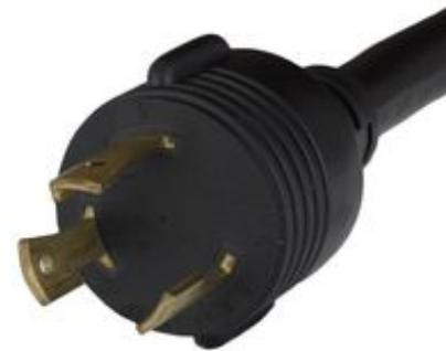
The NEMA 6-30P is a (hot-hot-ground) grounded plug that is rated up to 250V and 30A. This plug will supply either 208V or 240V based upon your electrical service, and will provide no neutral connection. This is commonly found on in-rack power distribution units where the electrical service is greater than 120V. The locking safety feature prevents this plug from disconnecting without intent
