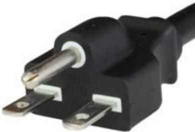
The NEMA 6-15P is a 3 Wire grounded plug featuring two blades and a ground pin, rated up to 250V AC and 15 Amps. The NEMA 6-15P has two, horizontal blades on the top of the plug spaced 23/32" center to center and a ground pin spaced between the two on the bottom of the plug. The NEMA 6 Series is commonly used with 208V and 240V circuits depending on your electrical service
