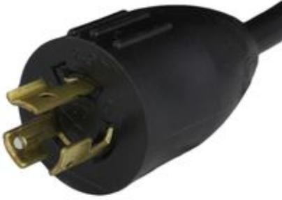
The NEMA L6-15P is a 3 Wire grounded plug with a hot, hot and ground pin rated up to 250V and 15A. This plug can be locked into place on the matching receptacle which prevents nuisance disconnection. The NEMA L6 Series is most commonly used for 208V or 240V applications, This plug can be distinguished by its tight pin alignment on the plug head and the outward turned tab on the ground pin.
