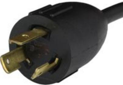
The NEMA L6-20P is a 3 wire grounded plug with a hot, hot and ground pin rated up to 250V and 20A. This plug can be locked into place on the matching receptacle which prevents nuisance disconnection. This plug is commonly found on in-rack power distribution units (PDU) where standard electrical service exceeds 125V, also in industrial settings to supply power to equipment or power tools.
