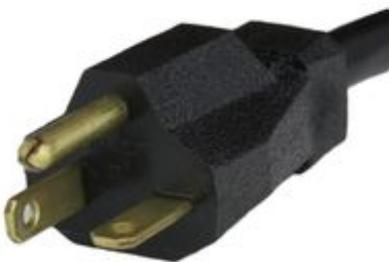
The NEMA 6-20P is a 3 Wire grounded plug featuring two blades and a ground pin, rated up to 250V AC and 20A. The 6-20P has a horizontal and vertical blade to prevent attachment to lower ampere rated receptacles. However, the 6-20R (receptacle) offers a "T" slot allowing connection of both a 6-20P and a 6-15P. Common applications are commercial ovens and large air condition units.
