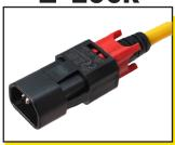
The Z-Lock is a universally locking power cord that locks on both ends of the power cord. The locking mechanism expands the body of the plug/connector by twisting the red plastic grip.
